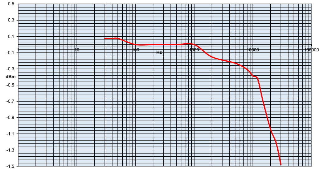
Frequency response, source: 0dBm, secondary loaded with 477R
