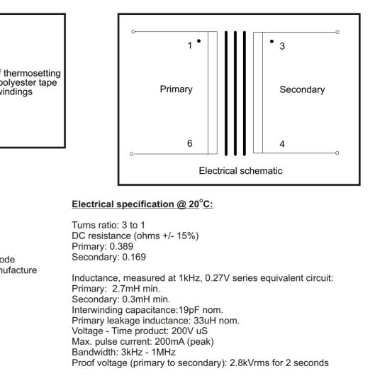
Operating temperature range: -40°C to +70°C Storage temperature range: -40°C to +125°C
