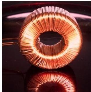
The high frequency choke ranges are based on low loss sendust powder cores. These have a saturation flux density three times higher than ferrite cores, and a distributed air-gap which gives a controlled hold-up of inductance with bias current.
